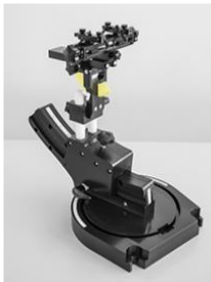
Device holder supplied by SPEAG
