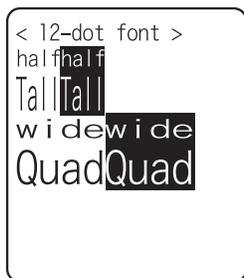
Test the function of LCD. When test starts the backlight turns ON automatically. However, when the Battery level is low it does not turn ON.
