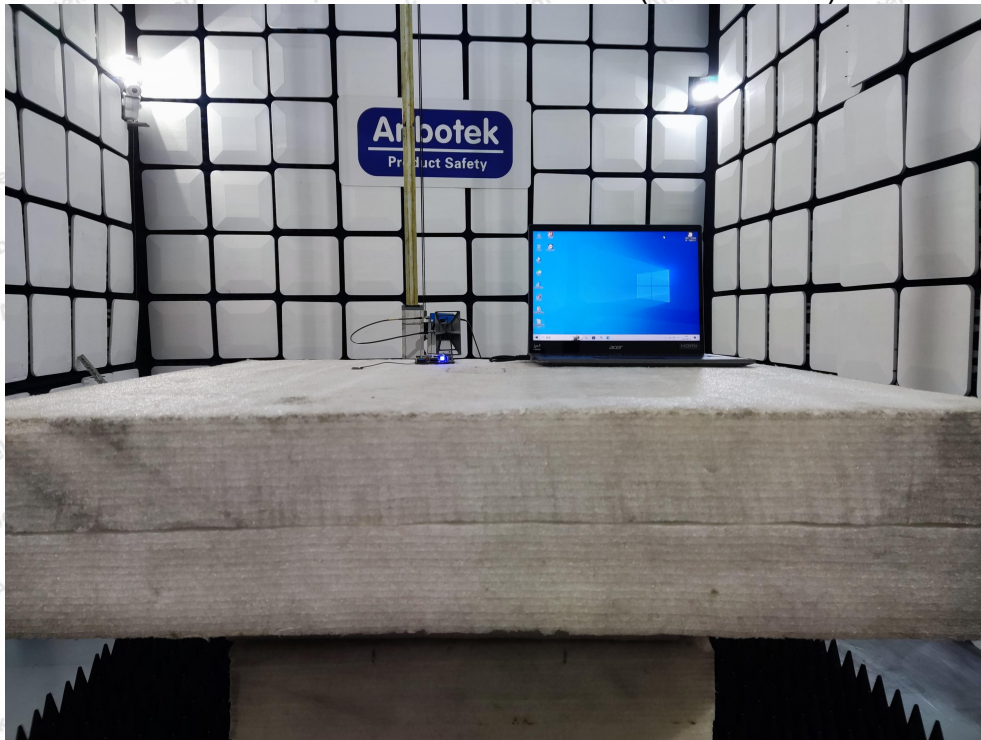
Photo of Radiation Emission Test (above 1GHz)
