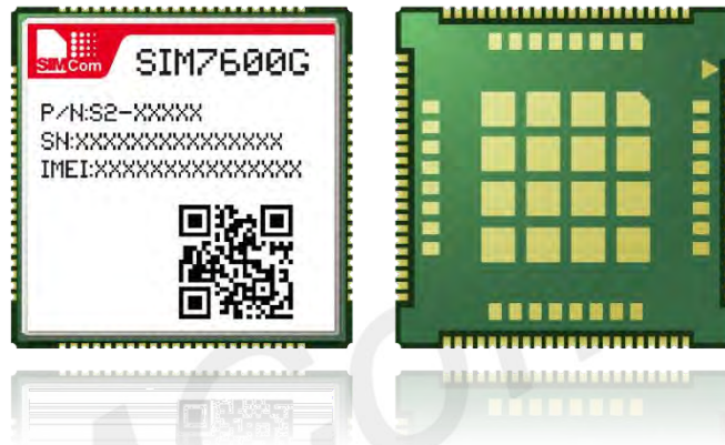
Figure 39: Top and bottom view of MODULE
