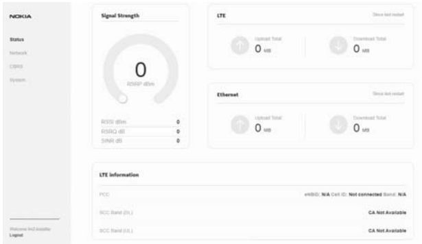
Figure 56 Example of the top part of the Status screen when the FastMile 4G Receiver is not connected to a cell
