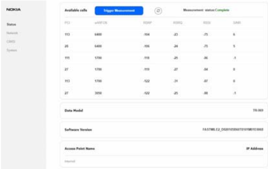
Figure 58 Example of the lower part of the Status screen with available cells when the FastMile 4G Receiver is not connected to a cell
