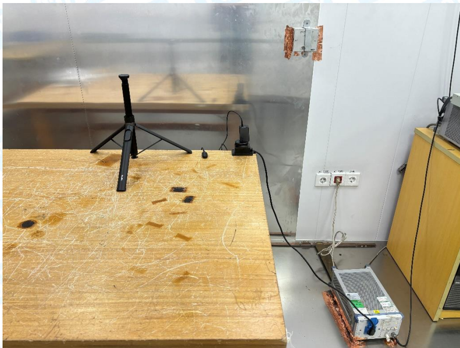
Photo of Setup for Conducted Emission
