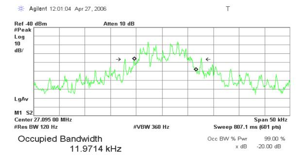
Transmit Freq Error619.950 Hzx dB Bandwidth14.863 kHz
