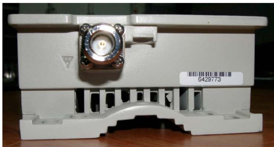
Photo # 4. Radio unit. RF & RJ45 connectors view
