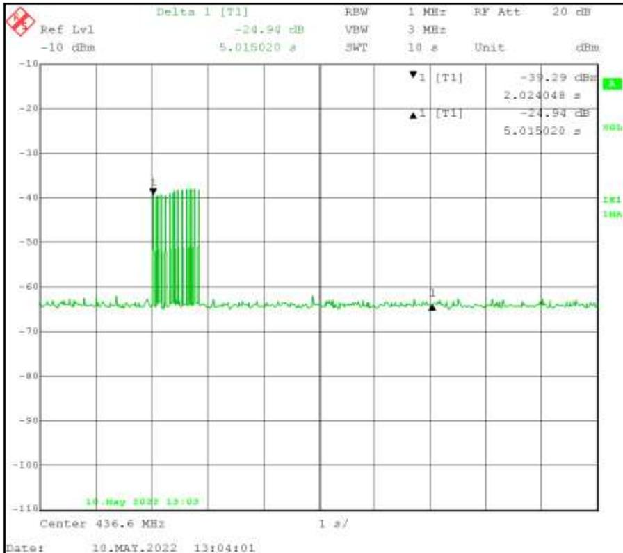
Test Results: The Lutron Model PD-6WCL Caseta RF Wireless Switch, BEC Sample #2204-01 complies with the 5 second deactivation requirements of 47 CFR Part 15.231 (a)(1) for Automatic Deactivation Measurement.
