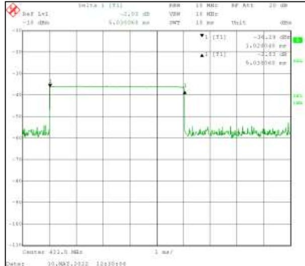
The measured on-times depicted on the spectrum analyzer screens above are used to calculate the Duty Cycle Correction Factor. This factor is used to reduce the emission level of spurious emissions measured and displayed in Section 4.3.
