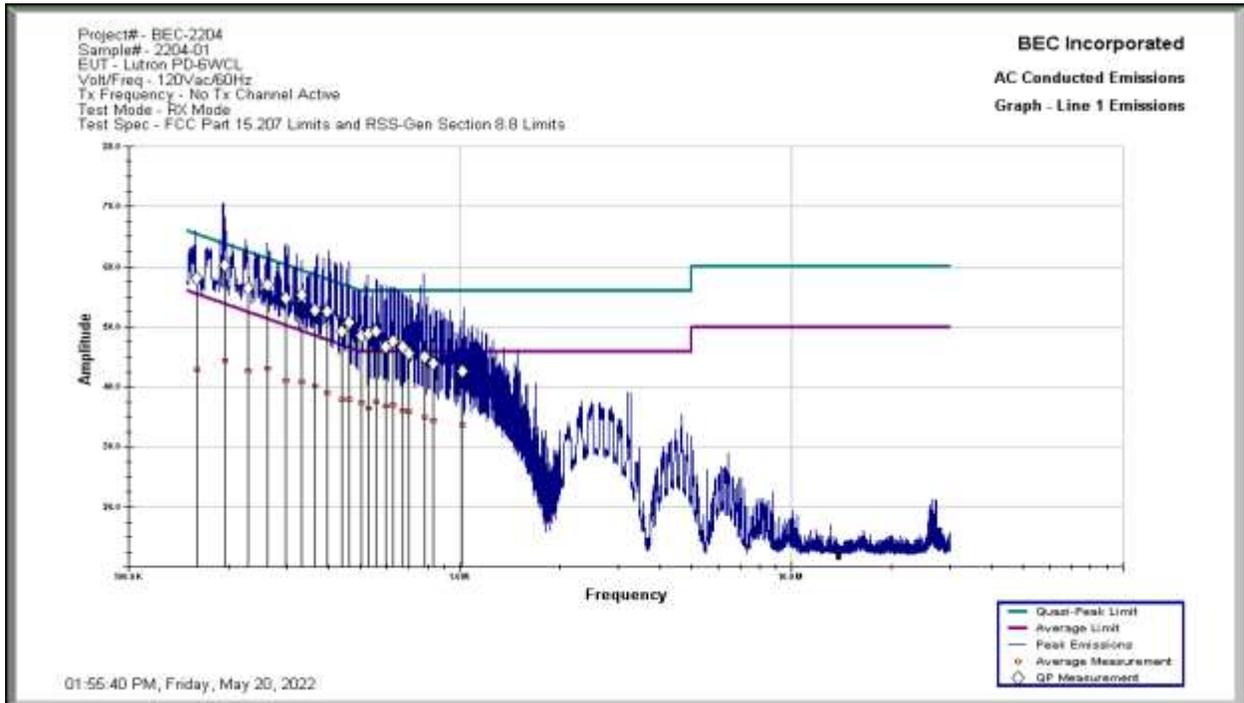
**Results:** The Lutron Model PD-6WCL Samples 2204-01 and 2197-02 comply with the requirements of FCC Part 15.207 and RSS-Gen Section 8.8. The margin is 1.17 dB @ 262.855 kHz with Sample #2204-01 transmitting Low Channel, 431.5 MHz, Neutral Line.
