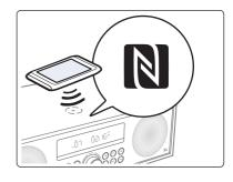
To disconnect, tap the mobile device on the NFC sensing area of the unit to disconnect or disable NFC from your mobile device.
