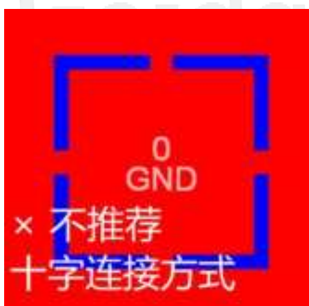
Figure 5.4 Unrecommended Copper Laying Connection
