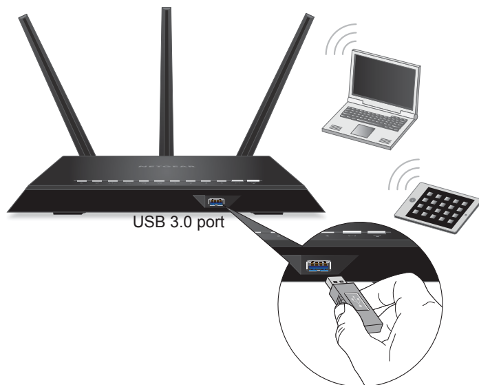
Figure 9. The blue USB 3.0 port on the front of the router provides the fastest access
