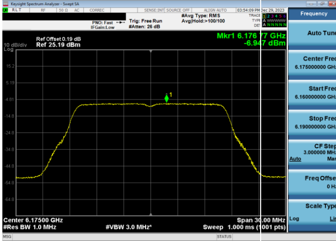
Plot 7-231. Power Spectral Density Plot Antenna WF7a Low Power Indoor (20MHz 802.11a (UNII Band 5) – Ch. 45, 24Mbps)
