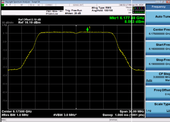
Plot 7-281. Power Spectral Density Plot Antenna WF7a Standard Power (20MHz 802.11a (UNII Band 5) – Ch. 45, 24Mbps)
