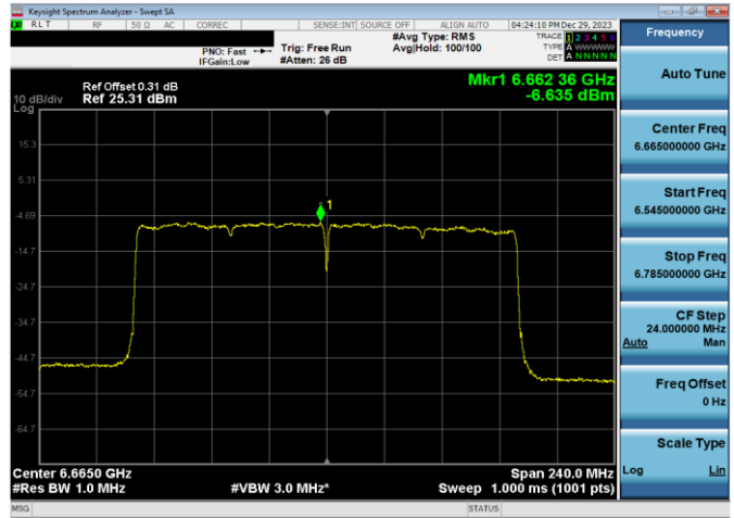
Plot 7-245. Power Spectral Density Plot Antenna WF7a Low Power Indoor (160MHz 802.11ax (UNII Band 7) – Ch. 143, MCS4)
