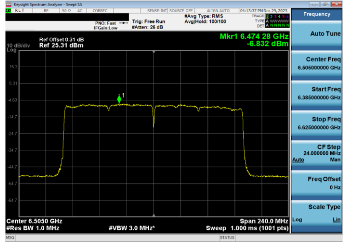
Plot 7-240. Power Spectral Density Plot Antenna WF7a Low Power Indoor (160MHz 802.11ax (UNII Band 6) – Ch. 111, MCS4)
