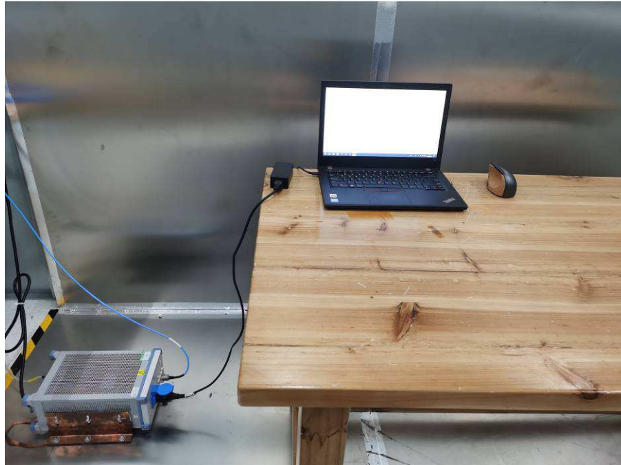
Photograph 3: Set-up for Conducted Emission on AC Mains
