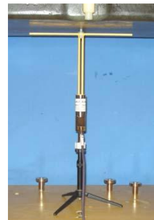
SPEAG 835 MHz Validation Dipole Setup
