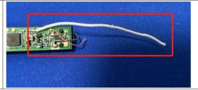
The antenna is internal antenna.
