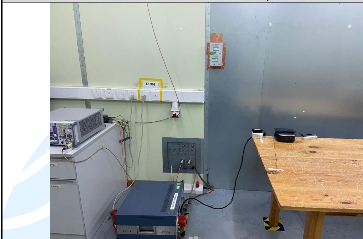
Conducted Emission Test Setup
