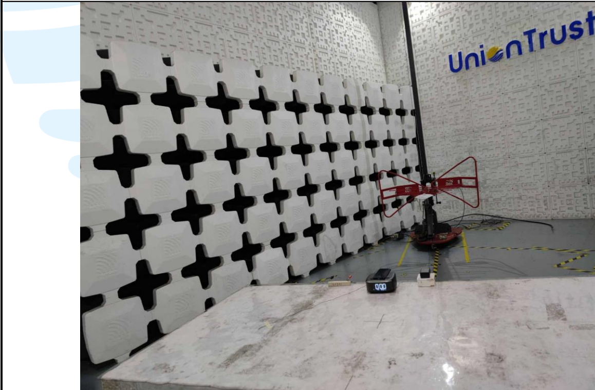
Radiated emission Test Setup (30MHz-1 GHz)
