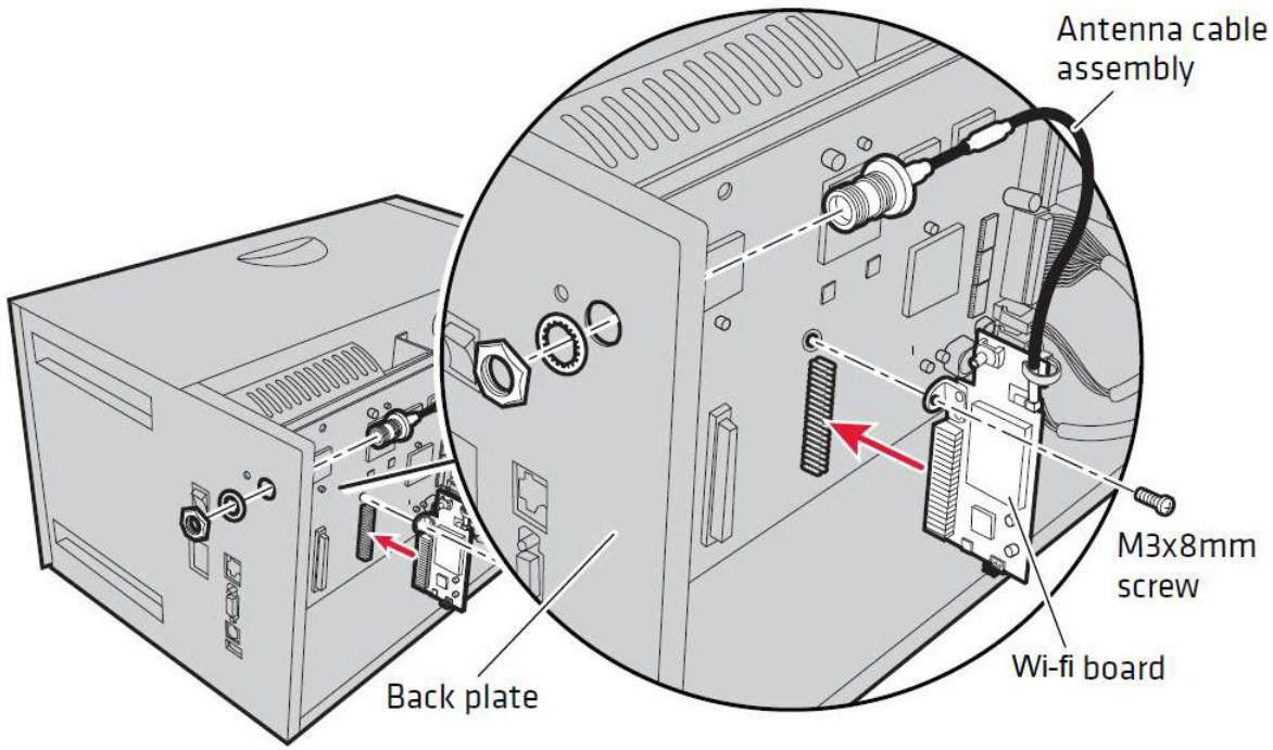
7. Install the other end of the antenna cable on the back plate and tighten the nut.
