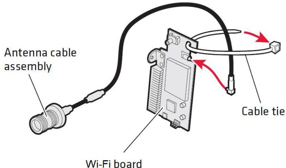
4. Secure the antenna cable to the Wi-fi board with a cable tie. Note the location of the head of the cable tie.
