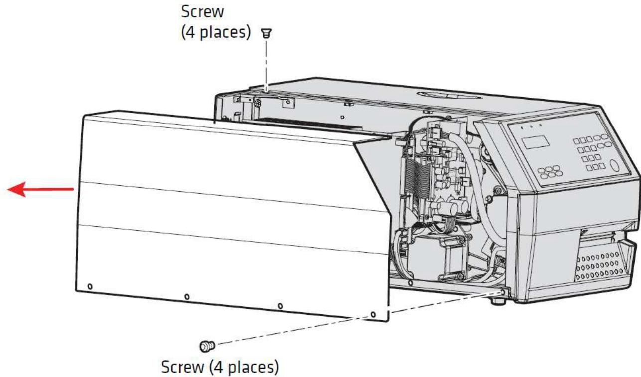
2. Put the cover aside on a soft cloth to avoid scratches.
