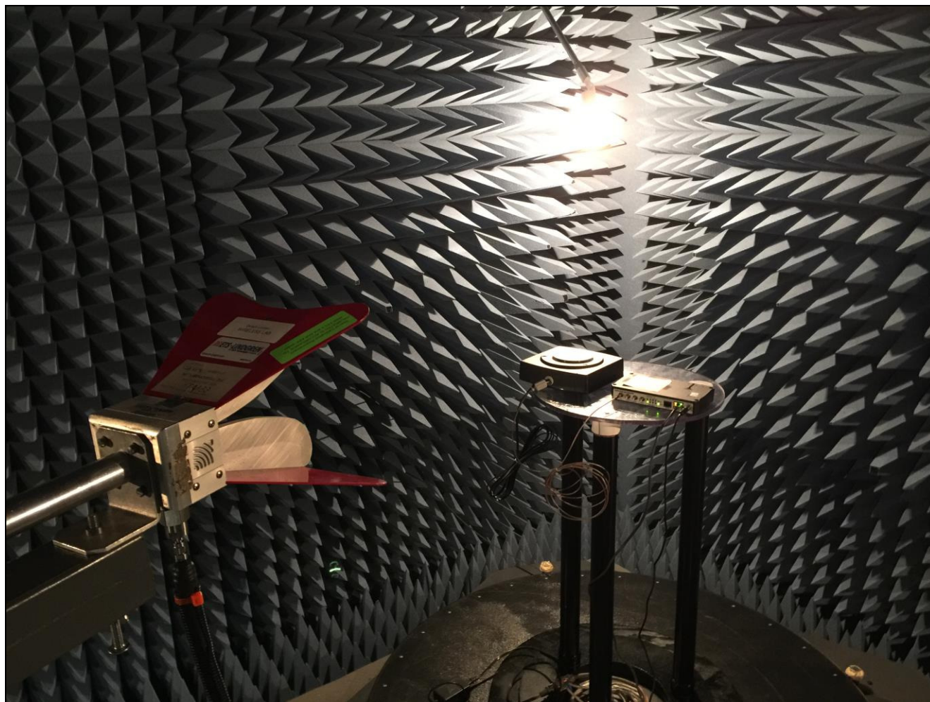
Photograph 1. Radiated Spurious Emissions, Test Setup
