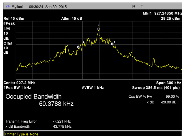
Plot 3. 20 dB Occupied Bandwidth, High Channel
