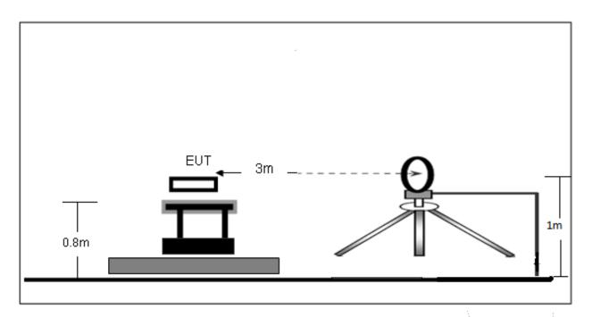
(B) Radiated Emission Test-Up Frequency 30MHz~1GHz
