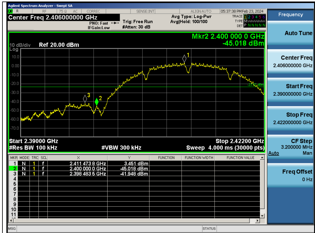
Test_Graph_802.11b_ANT2_2412_1Mbps_Lower Band Edge Emissions
