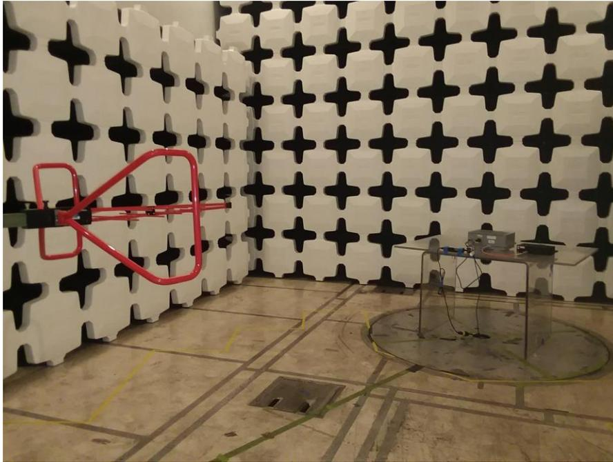
**Figure 2: Radiated Emissions, 30MHz – 1GHz Test Setup Photo**
