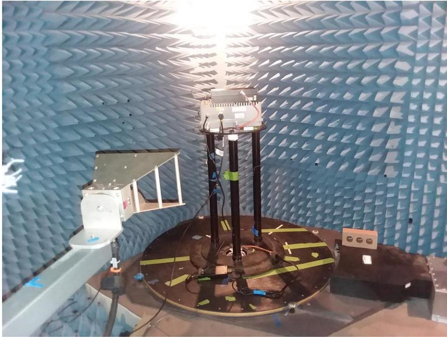
**Figure 3: Radiated Emissions, 1GHz – 18GHz Test Setup Photo**
