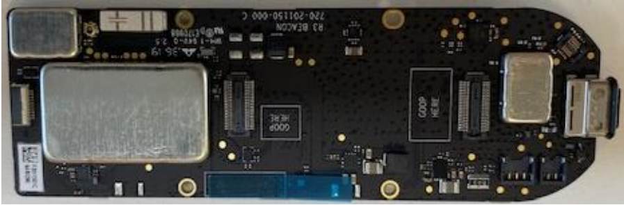
Beacon Main Logic Board Front Side with Shield Cans removed
