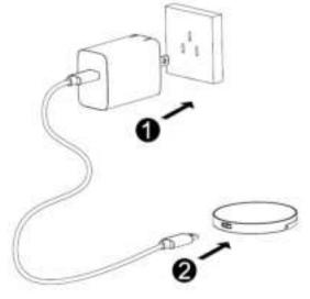
Use the supplied USB Type-C cable to connect a power adapter (not included) to the HTC Wireless Charger. Plug in your power adapter to an outlet.
