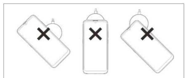
Make sure the back side of your phone (where the wireless charging coil is located) is placed on top of the HTC Wireless Charger. If your phone is not charging, adjust its position properly.
