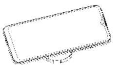
Place your Qi-compatible phone on top of the HTC Wireless Charger. Your phone will vibrate and charging will start automatically.
