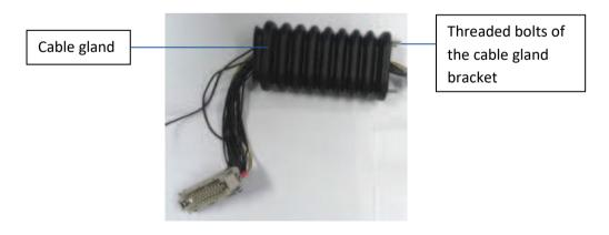
Fig. 52: Detached cable gland with bracket
