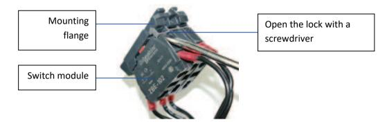
Fig. 44: Dismantling the auxiliary switch block
