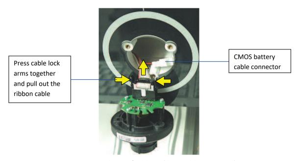
Fig. 49: Removing the rotary/push button (shown with battery removed)
