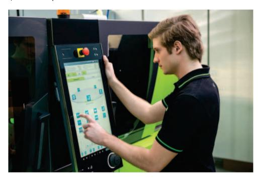
Fig. 29: CC300 Operator Panel installed in an industrial cabinet
