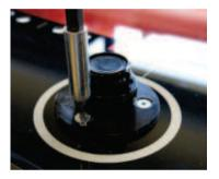
Fig. 47: Unscrew the cap holder of the rotary/push button
