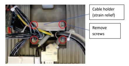
Fig. 51: Remove screws of the cable gland bracket
