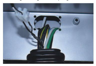
Fig. 32: Mounting the cable gland to the cabinet
