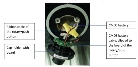
Fig. 48: Rotary/push button and CMOS battery, pulled out of the housing
