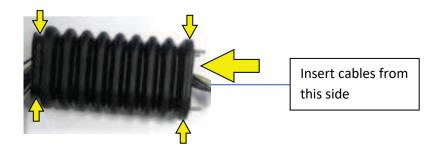
Fig. 55: Insert cables from the thicker end into the cable gland
