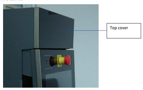
Fig. 36: Attaching the top cover of the CC300 cabinet
