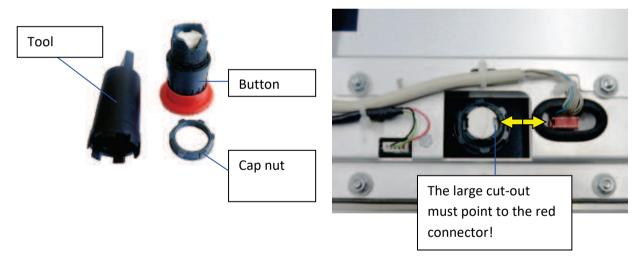
Fig. 43: Button of the emergency stop switch
