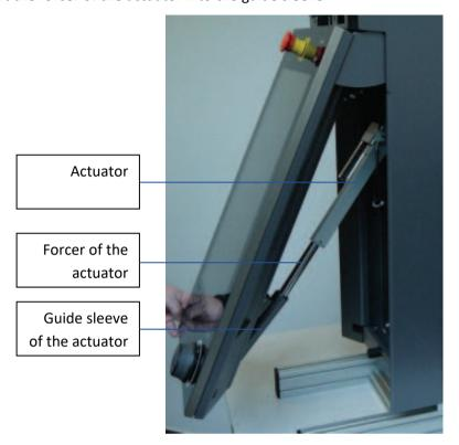
Fig. 35: Inserting the forcer into the guide sleeve of the actuator
