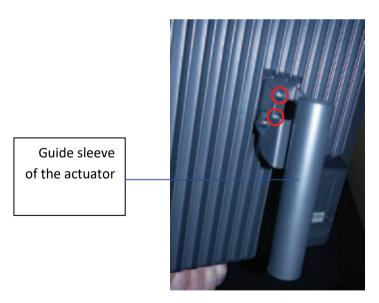
Fig. 34: Mounting the guide sleeve of the actuator to the CC300
