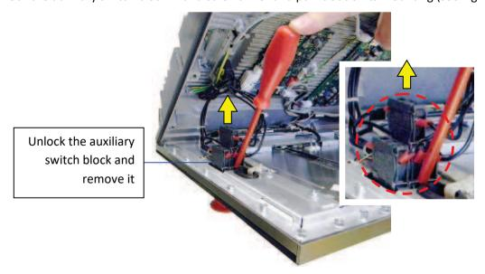
Fig. 27: Unlocking and removing the auxiliary switch block
