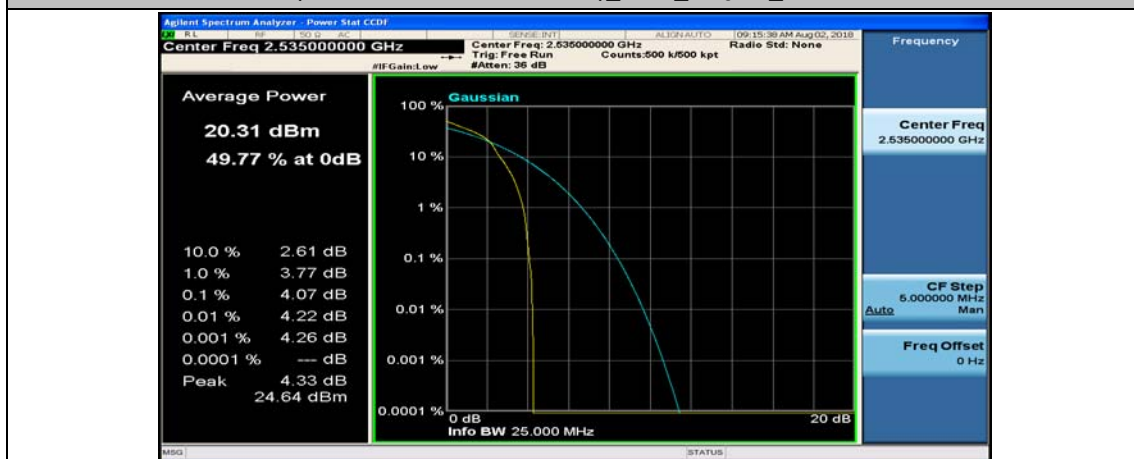
(Channel Bandwidth:15 MHz)_MCH_16QAM_1RB#37
