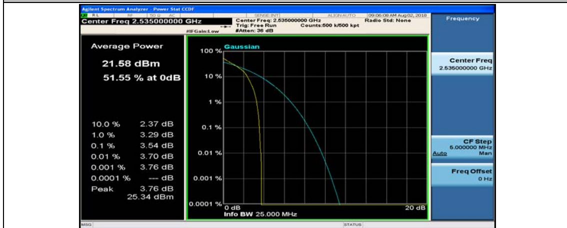
(Channel Bandwidth: 5 MHz)_MCH_QPSK_1RB#24
