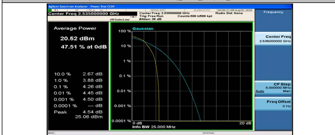
(Channel Bandwidth: 5 MHz)_MCH_16QAM_1RB#12
