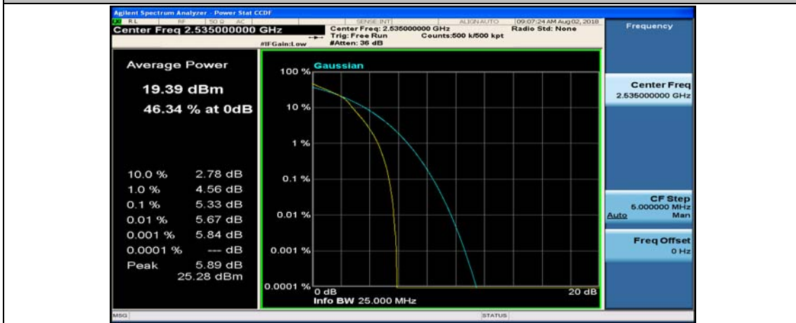
(Channel Bandwidth: 5 MHz)_MCH_16QAM_25RB#0
