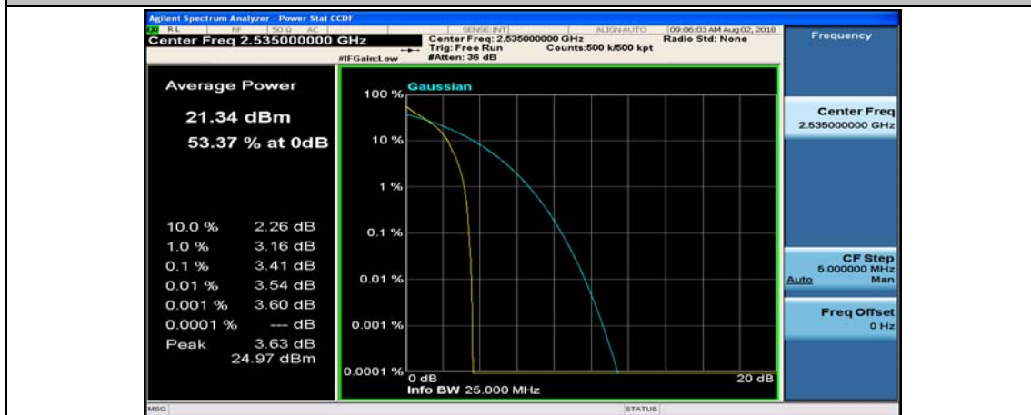
(Channel Bandwidth: 5 MHz)_MCH_QPSK_1RB#12
