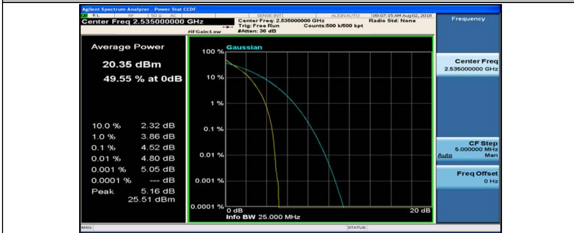
(Channel Bandwidth: 5 MHz)_MCH_QPSK_25RB#0
