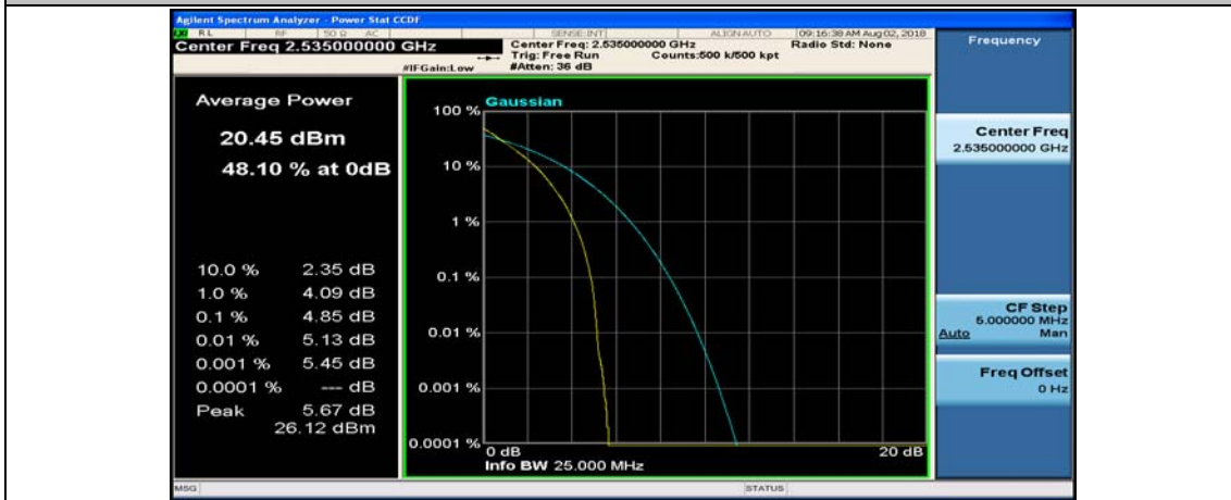
(Channel Bandwidth:15 MHz)_MCH_QPSK_75RB#0
