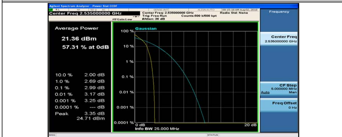
(Channel Bandwidth:15 MHz)_MCH_QPSK_1RB#37
