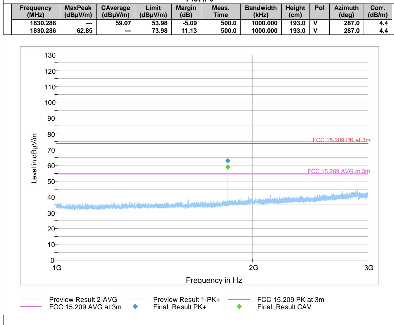
Note: 1830.286 MHz not within restricted bands of operation according to FCC 15.205.
