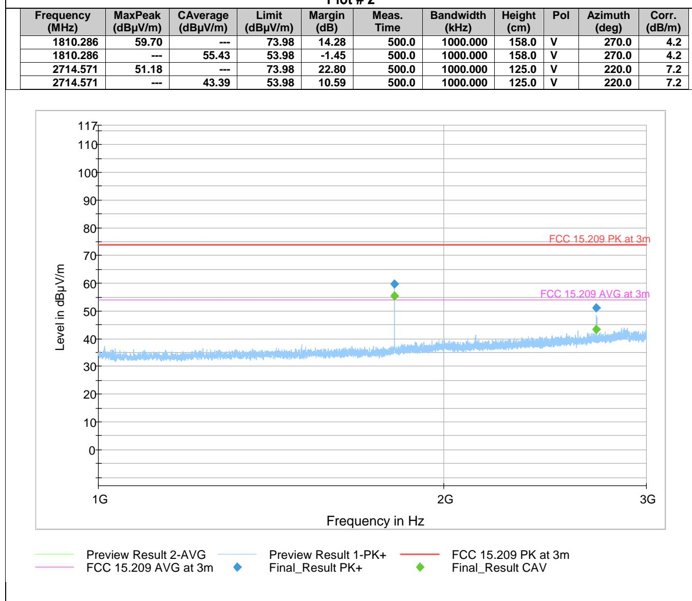
Note: 1810.286 MHz not within restricted bands of operation according to FCC 15.205.
