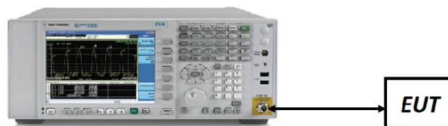
Figure 7-5. Test Instrument & Measurement Setup
