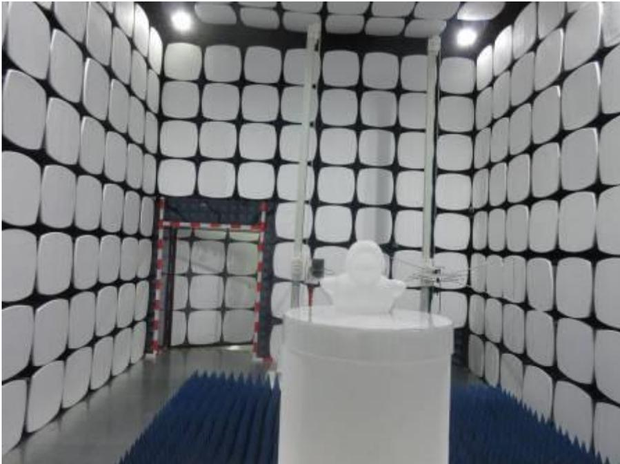
**1.3 Radiated Spurious Emissions Test Setup**
