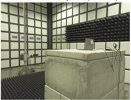
Radiated Emission Set up Photos (Above 1GHz)
