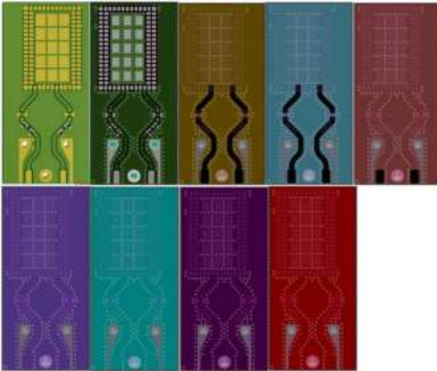
Figure 6: RF trace and ground design example
