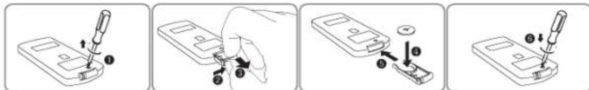
1. Loosen the screw with a screwdriver (not included) to open the battery compartment of the remote control.
