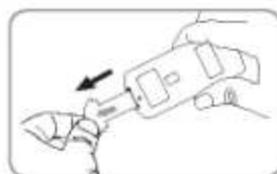
The unit has a pre-installed lithium CR2025 battery. Remove the protective tab to activate the remote control battery.
