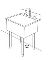
Note: If the surface you're placing on is not flat, try to place the sensor at the lowest point.
