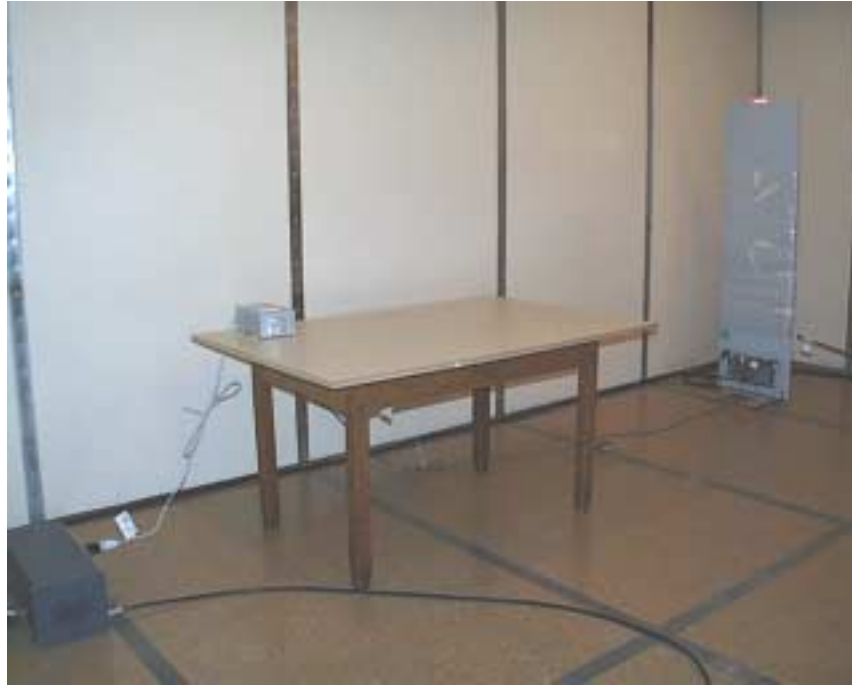
Photo 6 – Strata WX Conducted Emissions Test Setup
