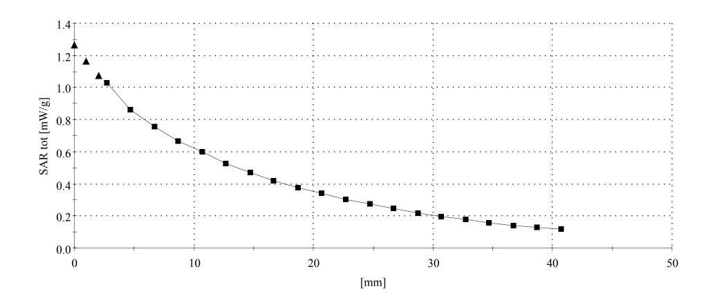
KWC-3245, 1900MHz Head, Right Cheek, PCS Ch600, Antenna Retracted, Z-Axis
