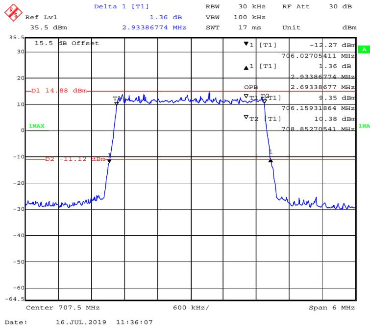
**QPSK (5 MHz) - 99% Occupied & 26 dB Emissions Bandwidth, Middle channel**
