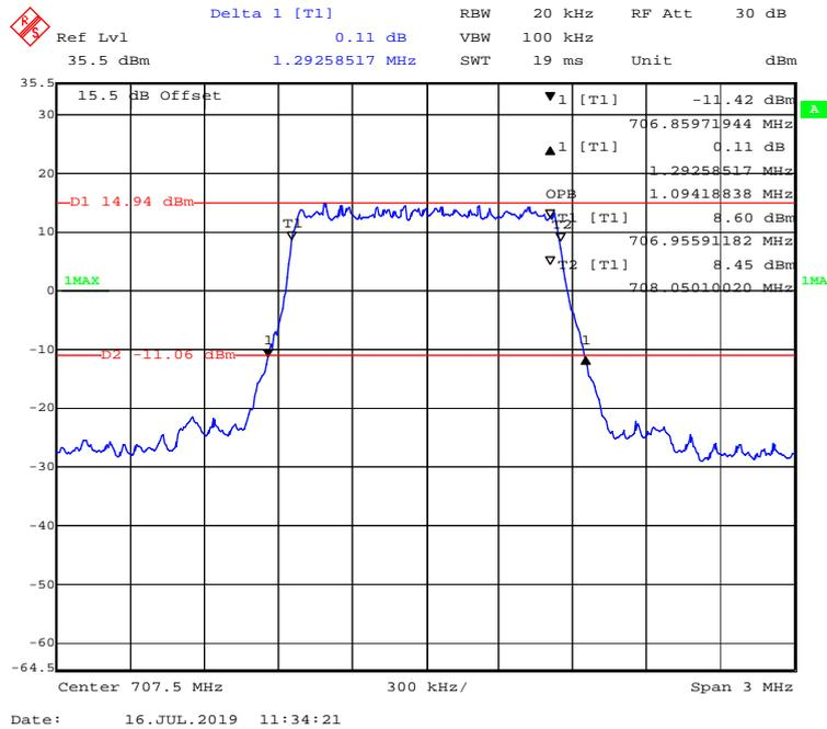
**QPSK (3 MHz) - 99% Occupied & 26 dB Emissions Bandwidth, Middle channel**
