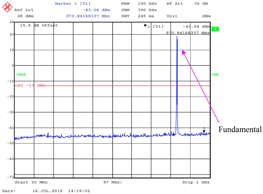
**1 GHz – 10 GHz (1.4 MHz, 16-QAM, Middle Channel)**
