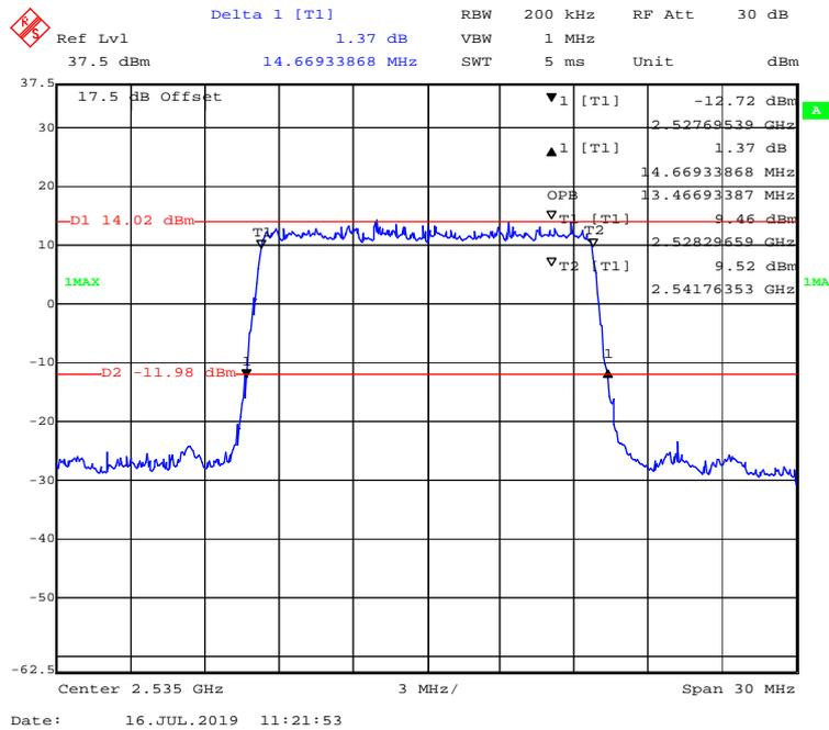
**QPSK (20 MHz) - 99% Occupied & 26 dB Emissions Bandwidth, Middle channel**
