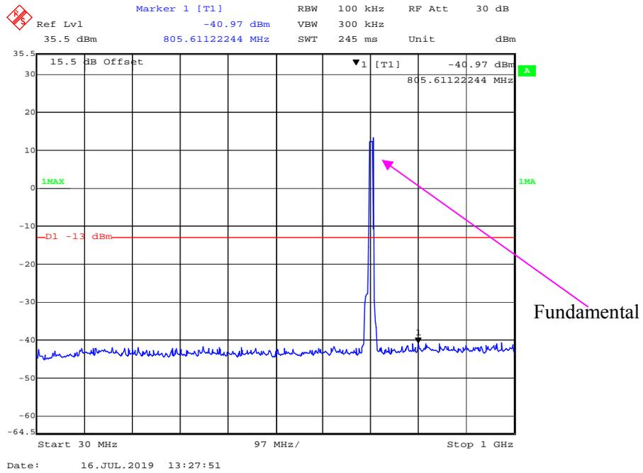
**1 GHz – 10 GHz (10 MHz, QPSK, Middle Channel)**
