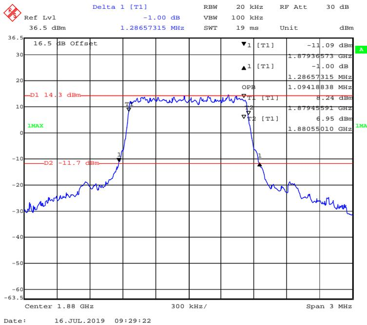
**QPSK (3 MHz) - 99% Occupied & 26 dB Emissions Bandwidth, Middle channel**
