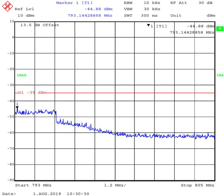
**793 MHz – 805 MHz, 10 MHz, 16-QAM**
