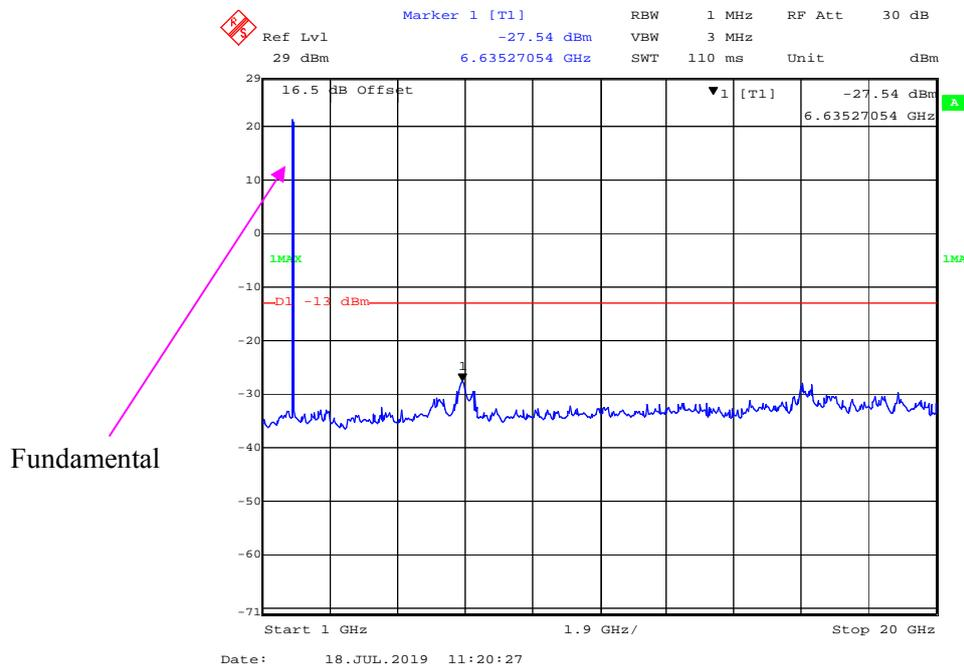
**30 MHz - 1 GHz (10 MHz, 16-QAM, Middle Channel)**
