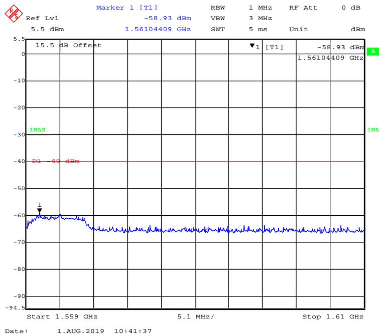
**1.559 GHz – 1.610 GHz (10 MHz, QPSK, Middle Channel)**
