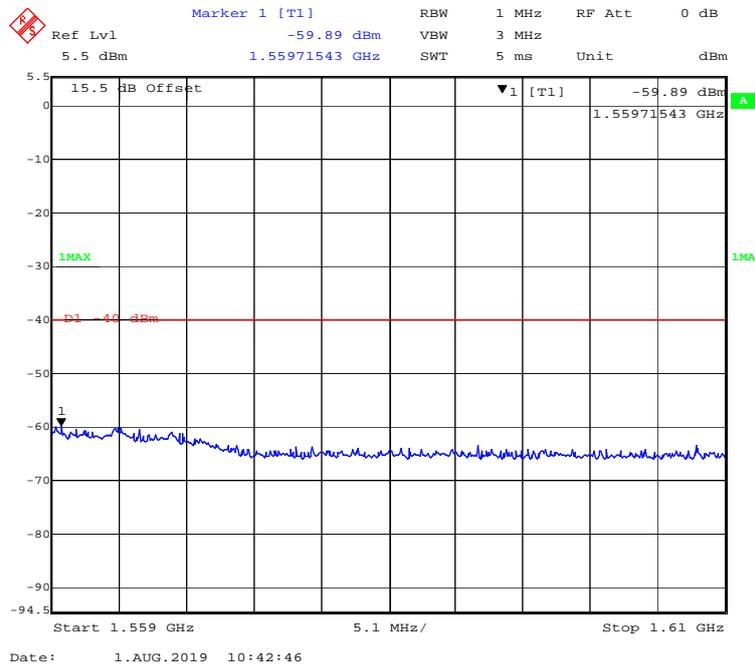
**1.559 GHz – 1.610 GHz (10 MHz, 16-QAM, Middle Channel)**
