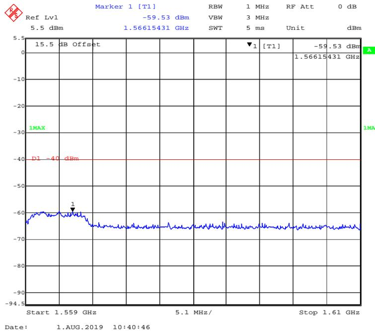
**1.559 GHz – 1.610 GHz (5 MHz, 16-QAM, Middle Channel)**
