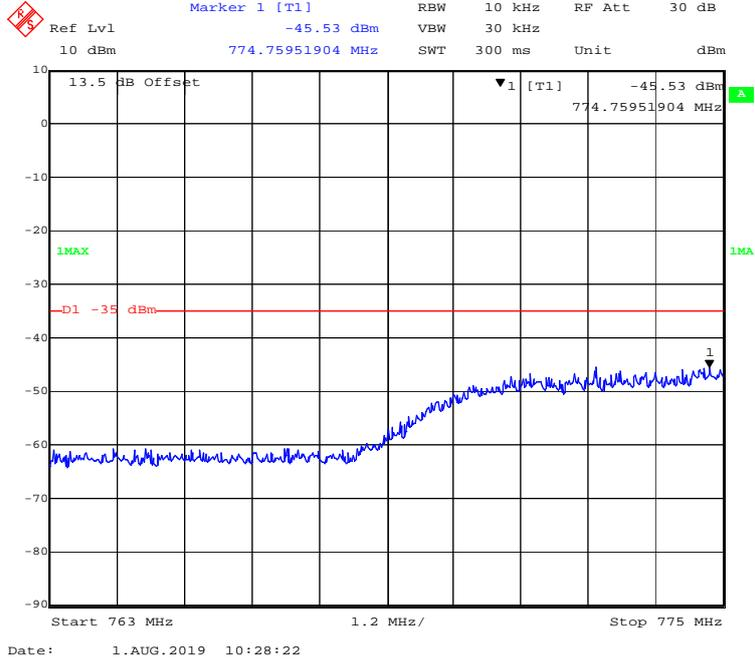
**763 MHz – 775 MHz, 10 MHz, 16-QAM**
