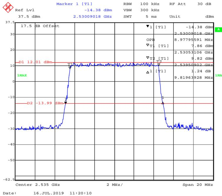
**QPSK (15MHz) - 99% Occupied & 26 dB Emissions Bandwidth, Middle channel**
