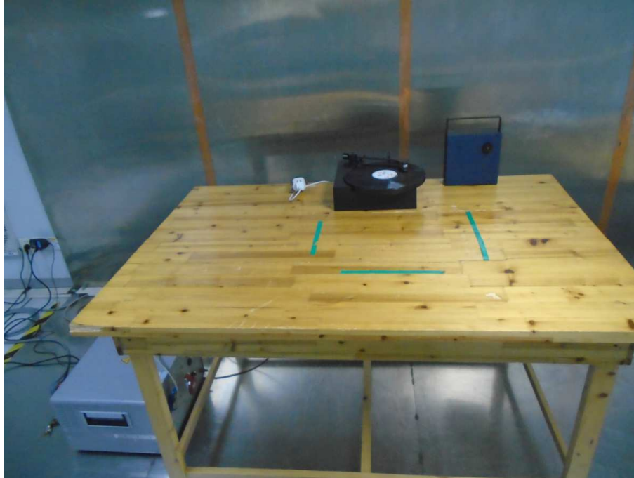
Photograph 1: Set-up for measurement of conducted emission
