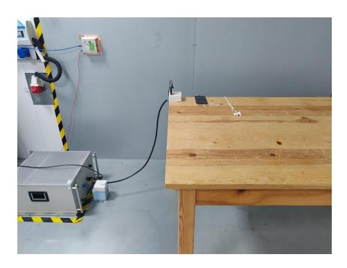
Set-up for Radiated Emission (RE), Below 1GHz
