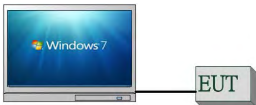
Fig. 2-1 Conducted Emission Configuration
