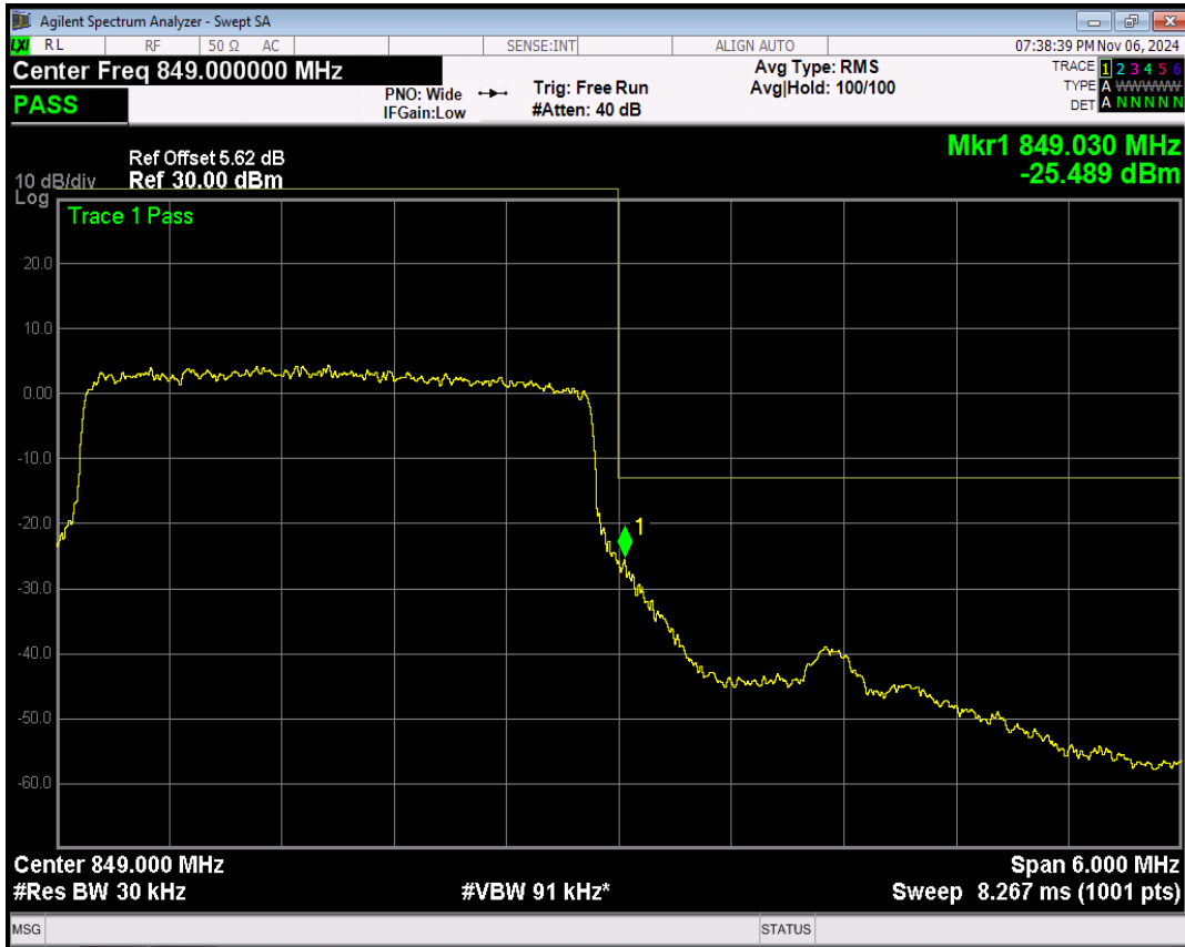
Band26(824-849) 16QAM BW=3MHz Channel=27025 RB Size=15 Position=#0
