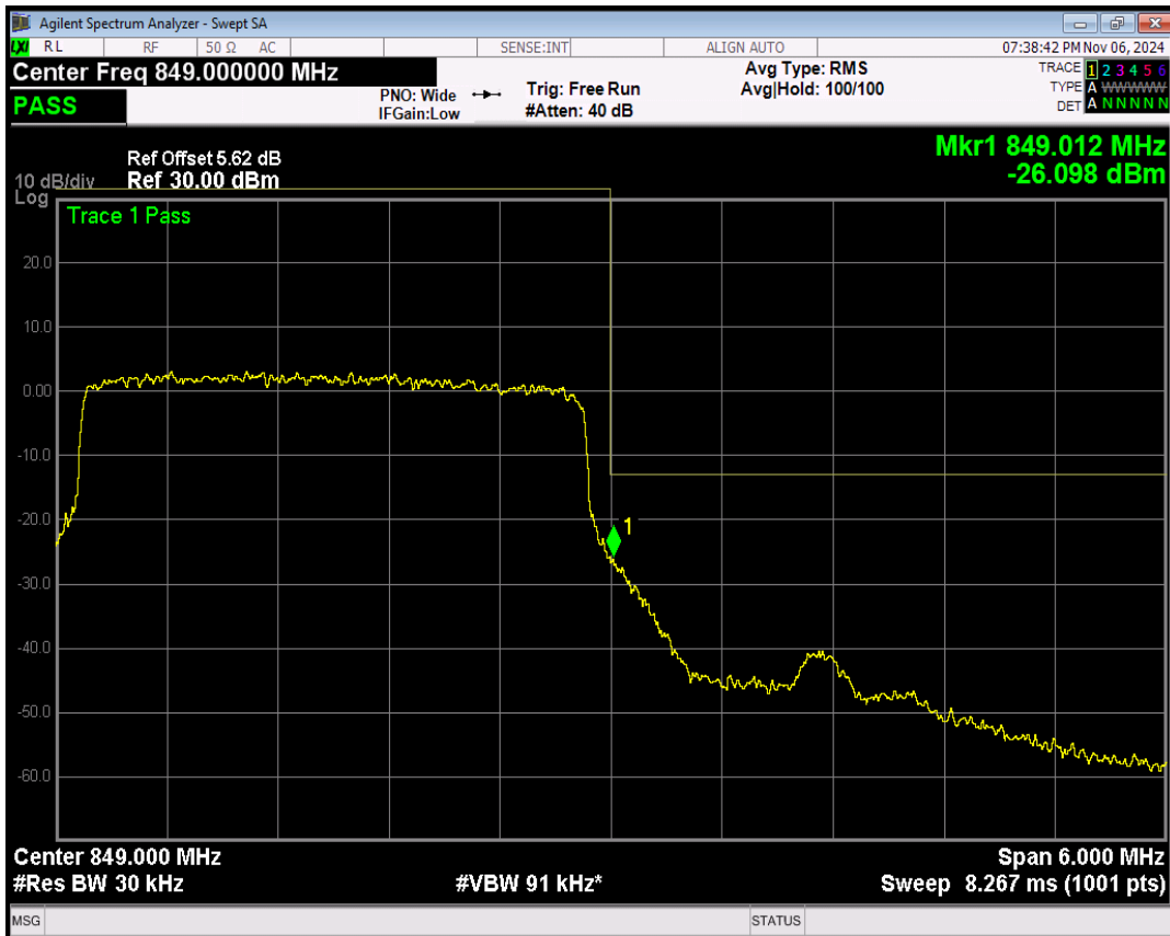
Band26(824-849) QPSK BW=5MHz Channel=26815 RB Size=25 Position=#0
