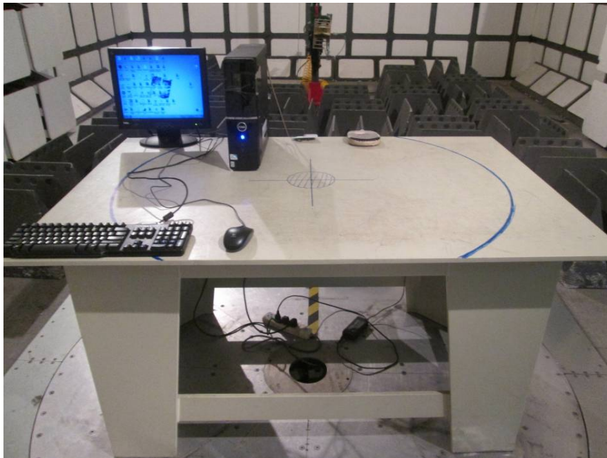
Radiated Emissions – Front View (Above 1 GHz)
