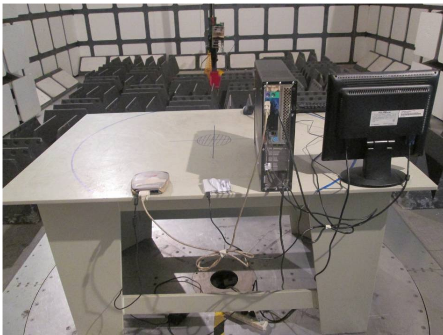
Radiated Emissions – Rear View (Above 1 GHz)
