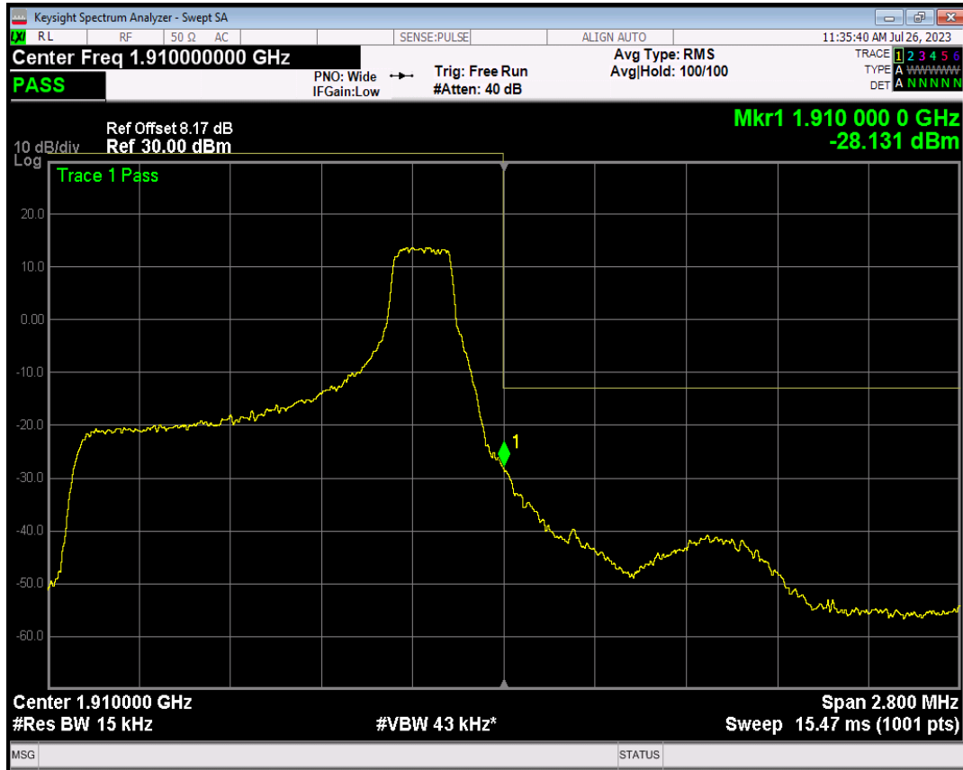
Band2 QPSK BW=1.4MHz Channel=19193 RB Size=6 Position=#0
