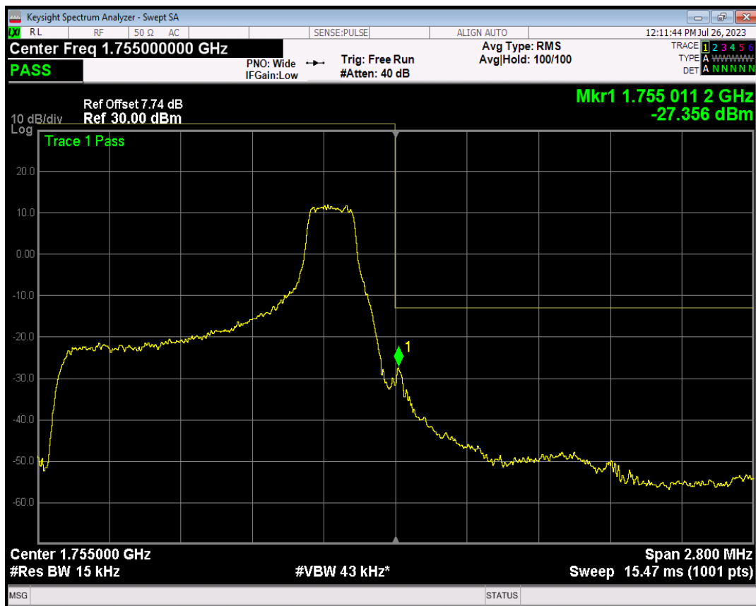
Band4 16QAM BW=1.4MHz Channel=20393 RB Size=6 Position=#0
