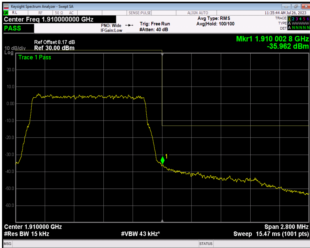
Band2 16QAM BW=1.4MHz Channel=19193 RB Size=1 Position=#0
