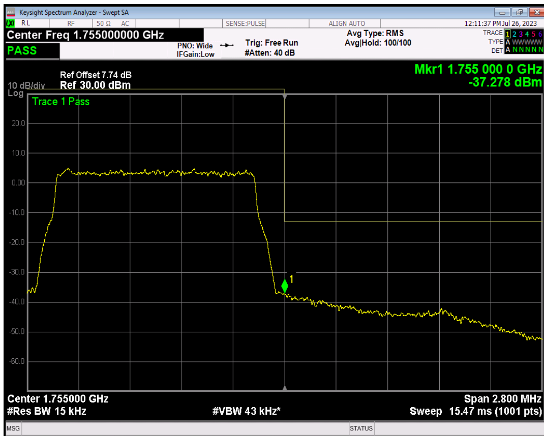
Band4 16QAM BW=1.4MHz Channel=20393 RB Size=1 Position=#0
