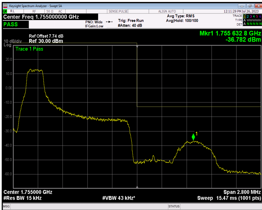
Band4 QPSK BW=1.4MHz Channel=20393 RB Size=1 Position=#Max
