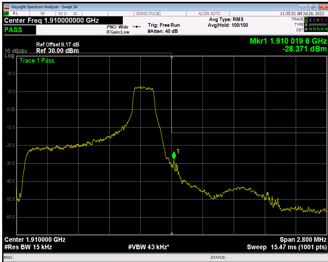
Band2 16QAM BW=1.4MHz Channel=19193 RB Size=6 Position=#0
