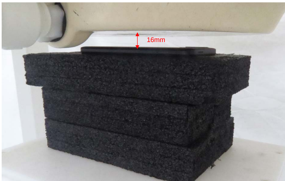
Picture 19: Back Side, the distance from handset to the bottom of the Phantom is 16mm
