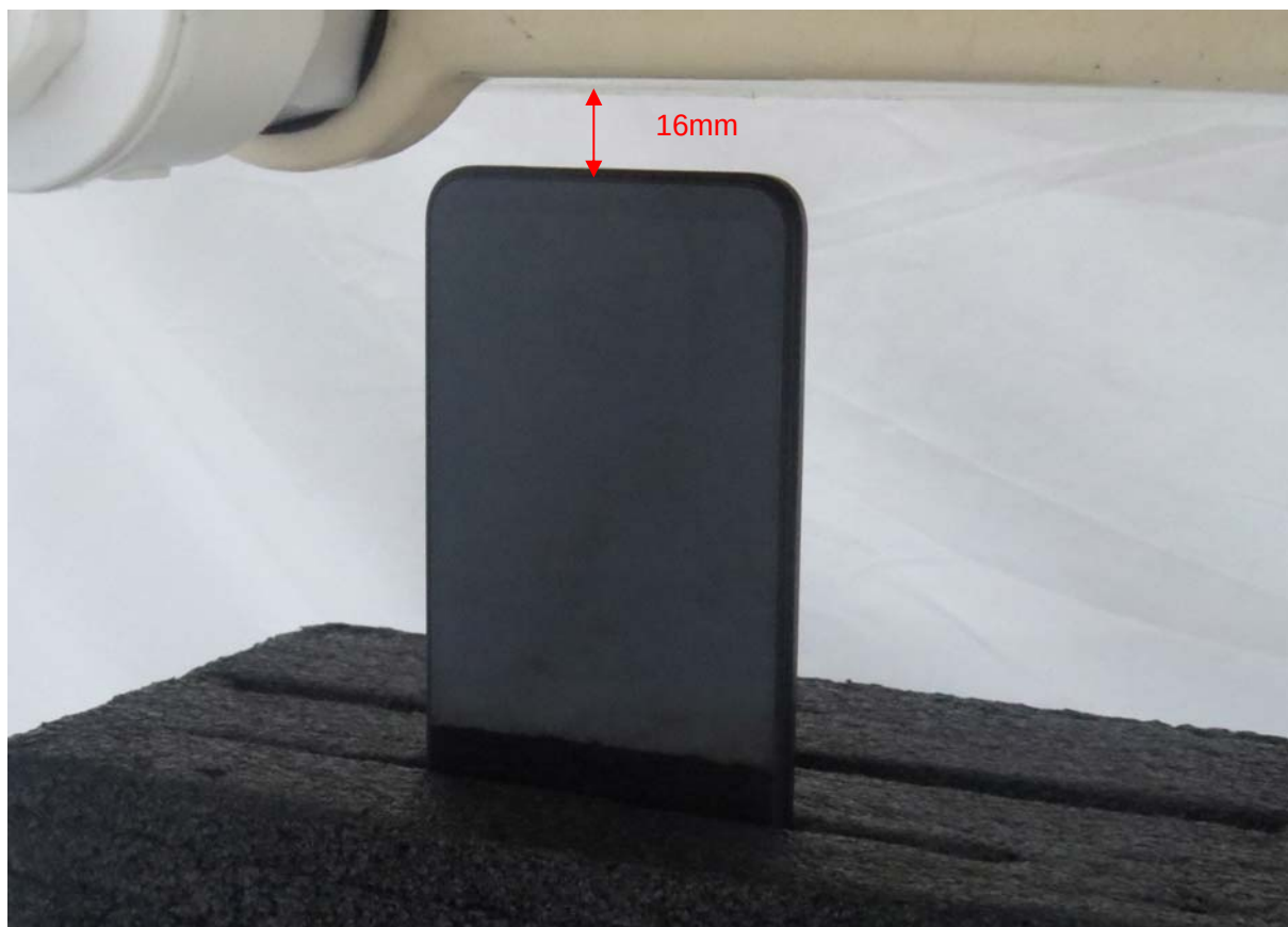
Picture 21: Bottom Edge, the distance from handset to the bottom of the Phantom is 16mm
