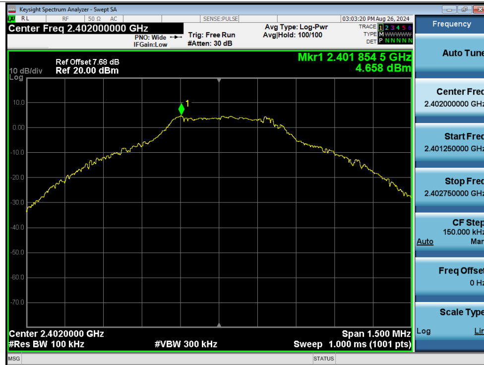
Tx. Spurious NVNT 1-DH5 2402MHz Ant1 Emission
