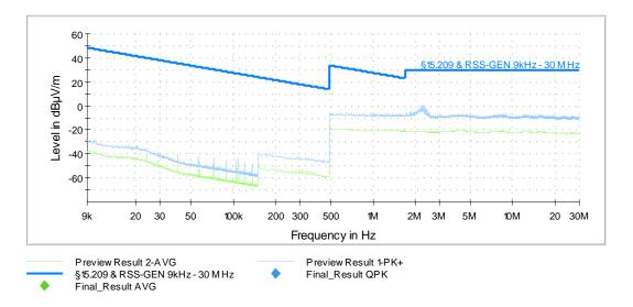
Remark: No emissions close than 20 dB to the limit, so no final measurement will be carried out.
