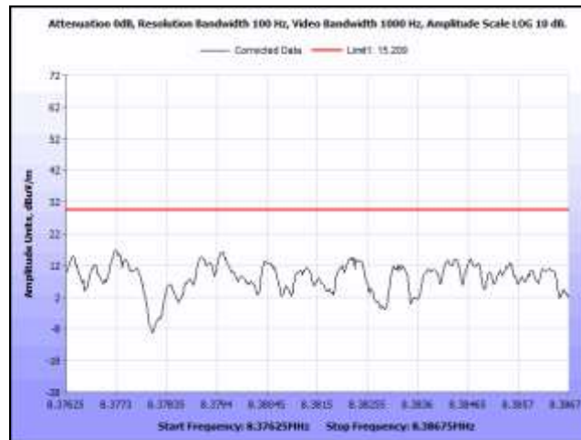
Plot 42. Radiated Restricted Band Edge, NP10, 8.37625 MHz – 8.38675 MHz
