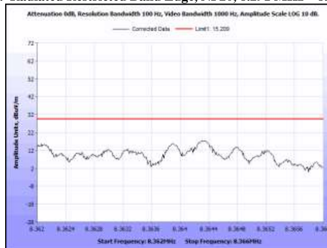
Plot 46. Radiated Restricted Band Edge, NP20, 8.362 MHz – 8.366 MHz
