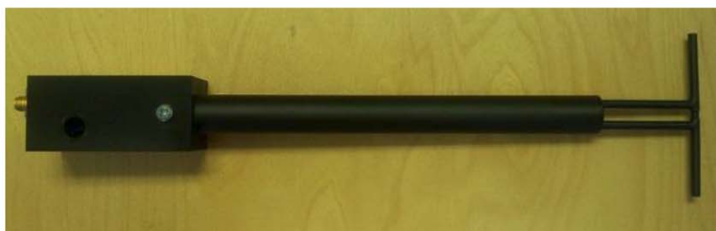
Figure 1 – MVG COMOSAR Validation Dipole
