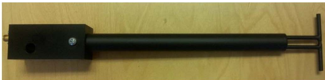
Figure 1 – MVG COMOSAR Validation Dipole
