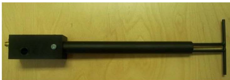
Figure 1 – MVG COMOSAR Validation Dipole
