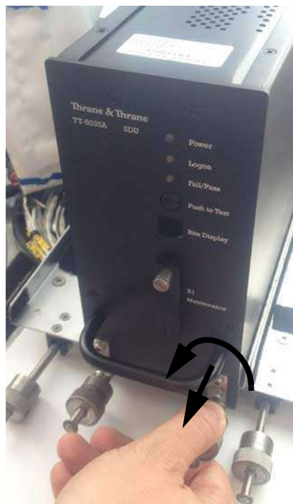
Figure 8-8: Exchanging an LRU (example)
