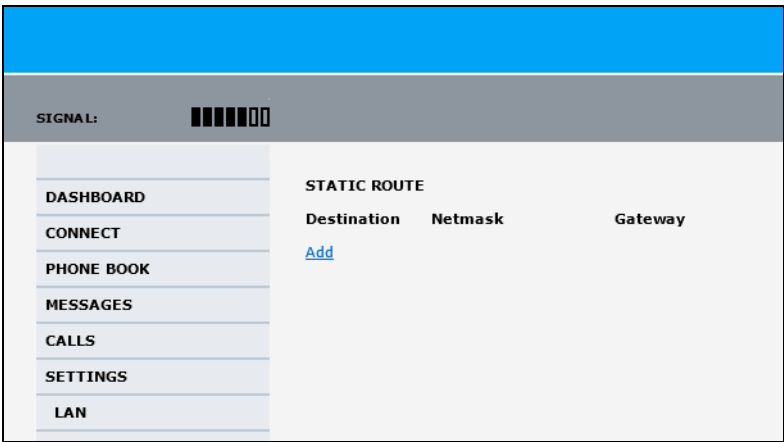
Figure 6-53: Web interface, Settings, LAN, Static route
