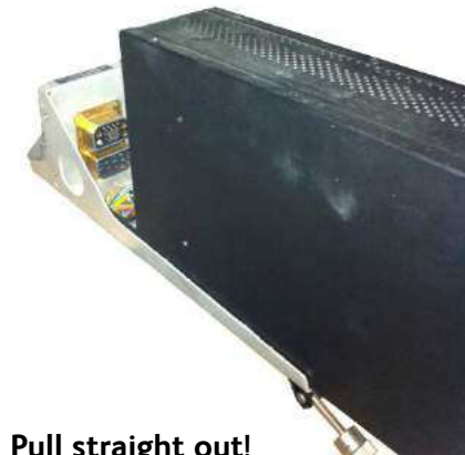
Figure 8-9: Pull out the LRU
