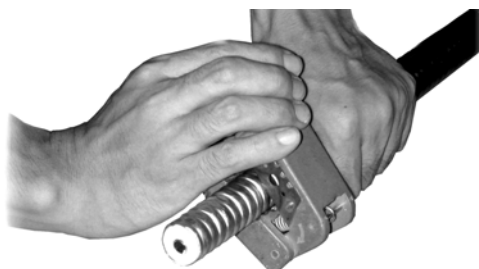
Fig. 10.4-7 Cutting the Feeder with a Cutter
