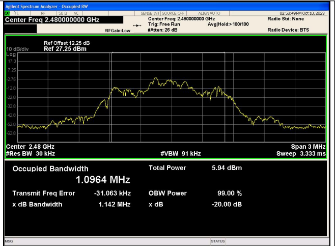
\pi/4 DQPSK 2-DH5_Channel 78
