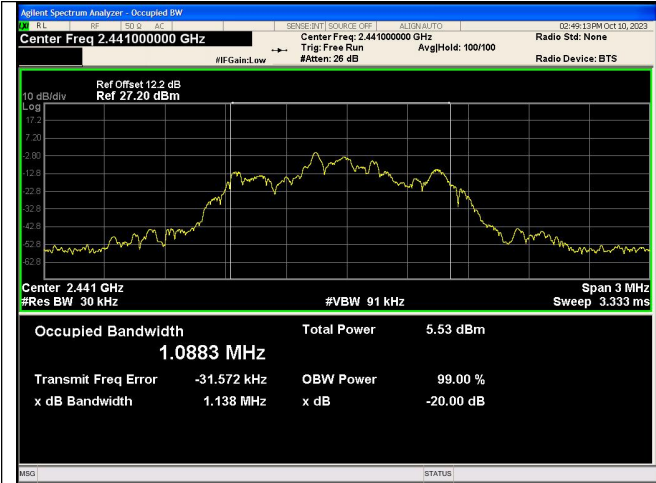
\pi/4 DQPSK 2-DH5_Channel 39
